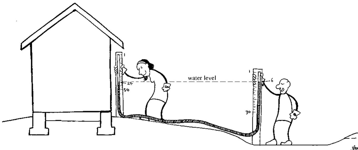
Fig. A1.6B. Using a bunyip to measure how much lower the bottom of the basin is than the area near the house, confirming that the slope now drains away from the house
