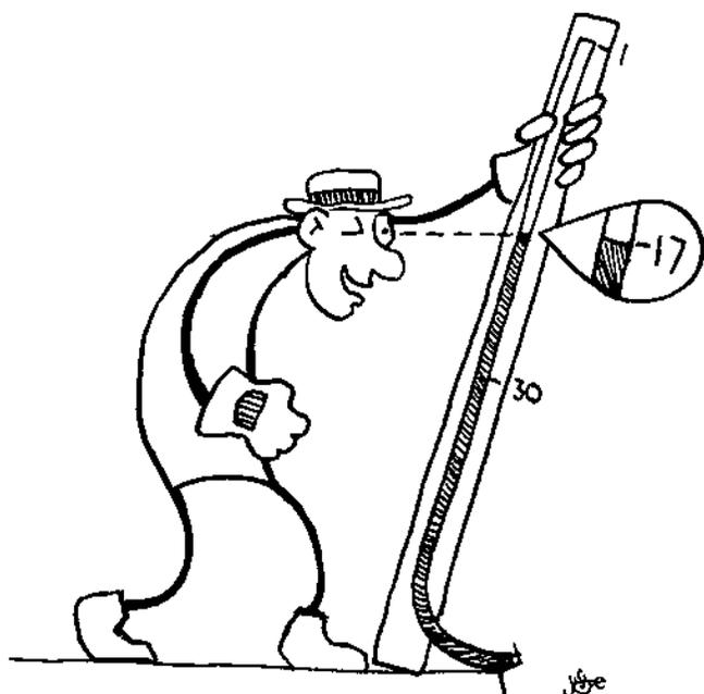
Fig. A1.4A. A non-vertical buniyip stake will give a lower, incorrect reading
