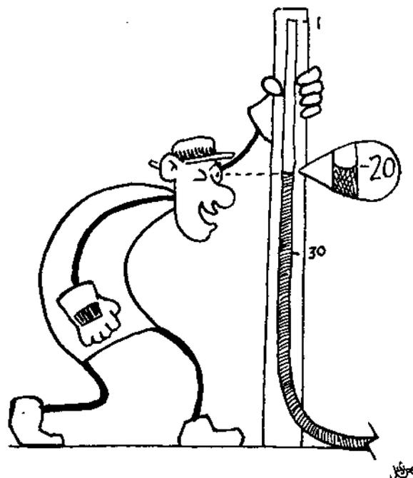
Fig. A1.4B. The buniyip stake must be vertical for a correct reading
