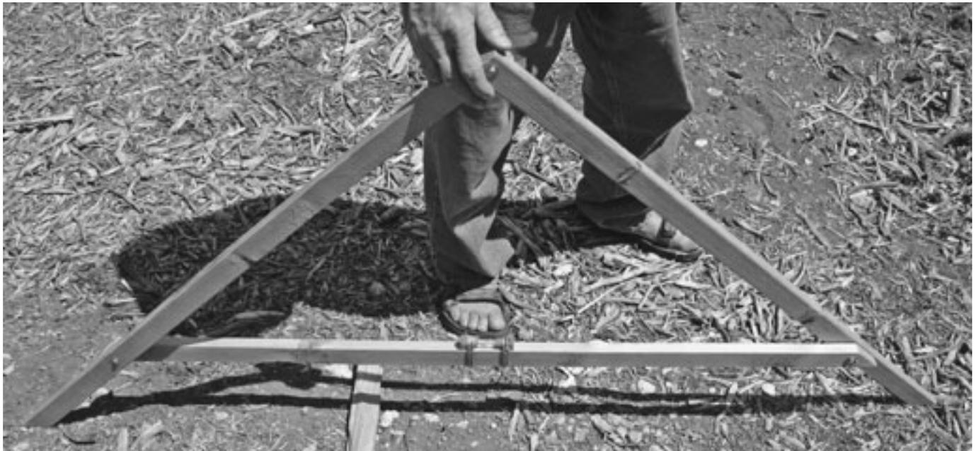
**Fig. A1.10.** Chris Meuli’s line-level A-frame. A bubble level tool is lashed to horizontal bar below Chris’ toes. Chris bolts his A-frame together with wing nuts so he can disassemble and fold it up for easy storage. His A-frame is only as tall as his waist, which allows him to use the tool under the branches of trees.
