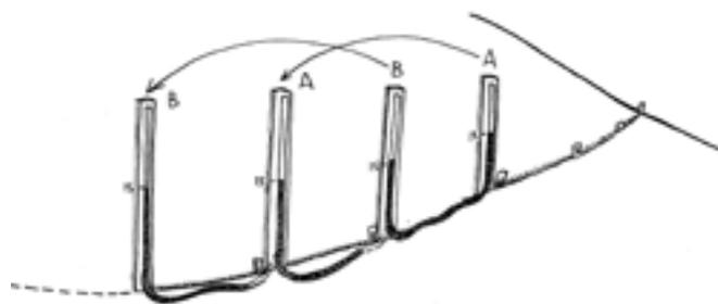
Fig. A1.5. Leapfrogging the buniyip to mark a level contour line on the land. Here the contour line is marked both by scuffing a line in the dirt and with stakes.
